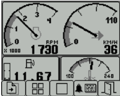
Figure 2. The Engine Monitor's top level button bar menu: Key 1: Pages icon indicating that further presses cycle through options for the screen being viewed (in this instance fuel computer modes for the main engine display) Key 2: Quad Display mode Key 3: Uni Display mode Key 4: Alarm Display mode Key 5: Exit door
