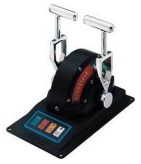
The 6508 is illuminated, but not water tight. This unit must be protected from the elements. The 6508 can be equipped with two potentiometers per handle. This will give redundancy in the electronic control system. The microprocessor will read the two potentiometers at all times and if the microprocessor considers one of them defective, it will ignore it and read the intact potentiometer only.
