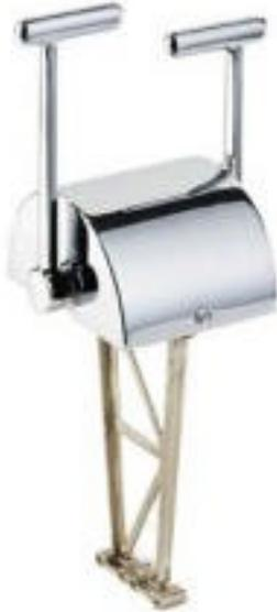
This control is available with three different handles; standard, handles with plastic grips or curved handles with knobs. An optional clutch and throttle interlock can be ordered with this unit. The purpose of this interlock is to prevent shifting, above engine idle. It is only available for systems having clutch and throttle on the same control. In two station applications only one interlock is required. For gears with an electric clutch, an adapter with two microswitches can be ordered.
